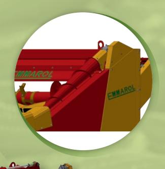
**Side snap rolls** are standard equipment of every machine. They make it easier to work in the field with tilted and laying corn. The rolls are driven by means of V-belts with a maintenance-free tensioner. In order to facilitate access to working elements during machine servicing, the side cover of the header is lifted with aid of a gas cylinder.
