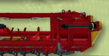
The header is driven from both sides of the machine. PTO shafts transmit the revolutions to a chain transmission equipped with a maintenance-free tensioner. Free access to chain wheels enables easy change of gear ratio, according to customers' requirements. The upper chain wheel mounted on the adjustable bracket allows you to adapt the drive to any combine.
